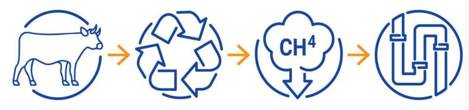
Capture biowaste from dairies, farms, food waste, landfills and waste water treatment plants Convert into biogas (anaerobic digestion, etc.) Process the biogas to make it pipelineready (biomethane)
